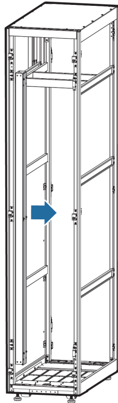
Figure 3-63 Removing the cable trough cover
