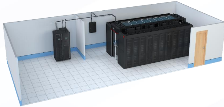
UPS Outside the Module(Smart Busway)
