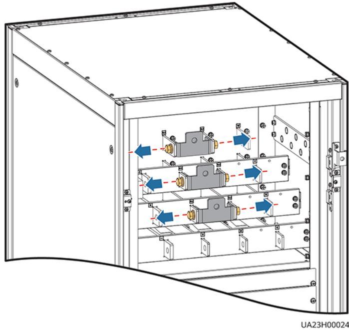
**Figure 3-108** Connecting power cables
