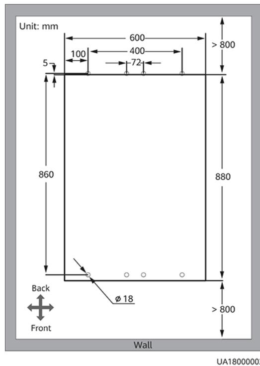
**Step 2** Drill holes for installing expansion bolts, and install expansion bolts.
