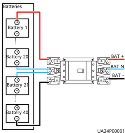
**Figure 3-72** Connecting power cables 2
