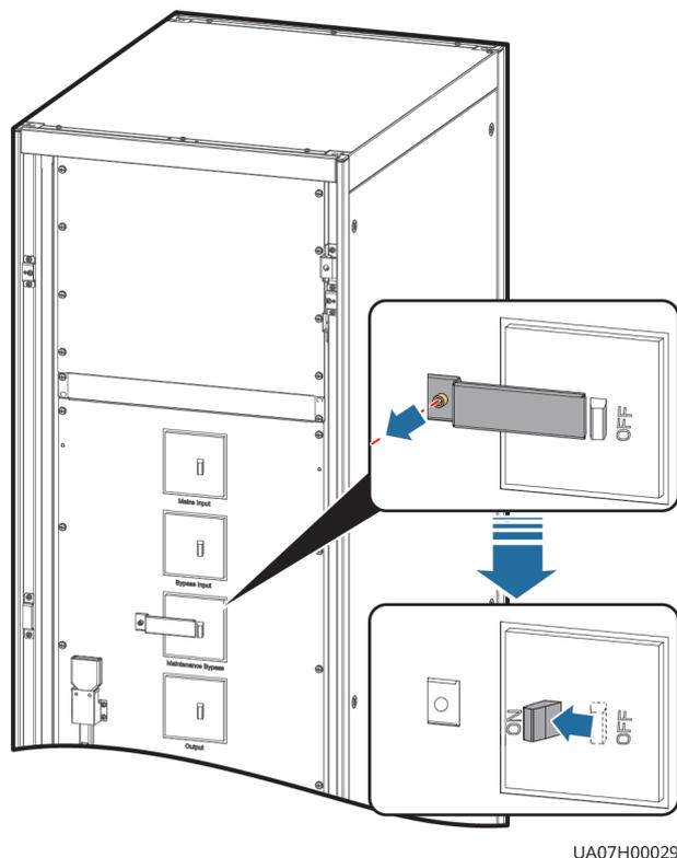
**Figure 8-4** Turning on the maintenance bypass switch (UPS5000-E-300K-SM)
