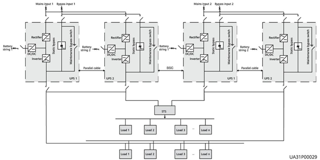
**Figure 3-118** Cable connections for a dual-bus system
