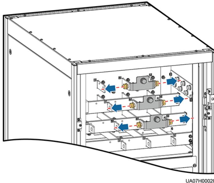
**Figure 3-70** Connecting power cables 1
