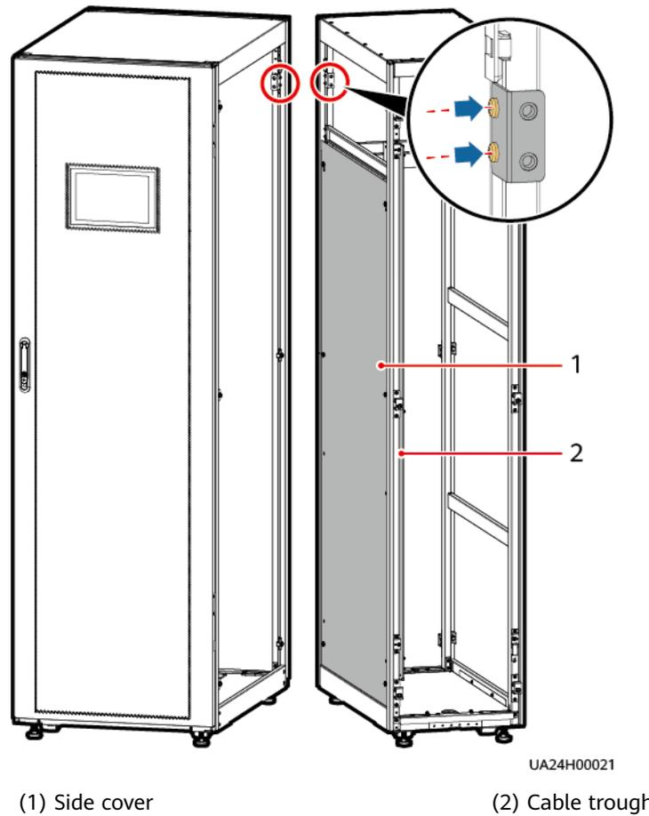
**Step 5** Place the cable entry cabinet on the right of the UPS cabinet.
