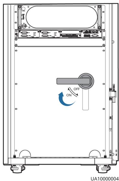
**Figure 8-5** Turning on the maintenance bypass switch (UPS5000-E-300K-SMT)
