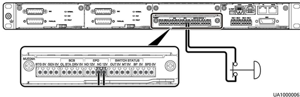
**Figure 3-112** Cable connection for an NO EPO switch
