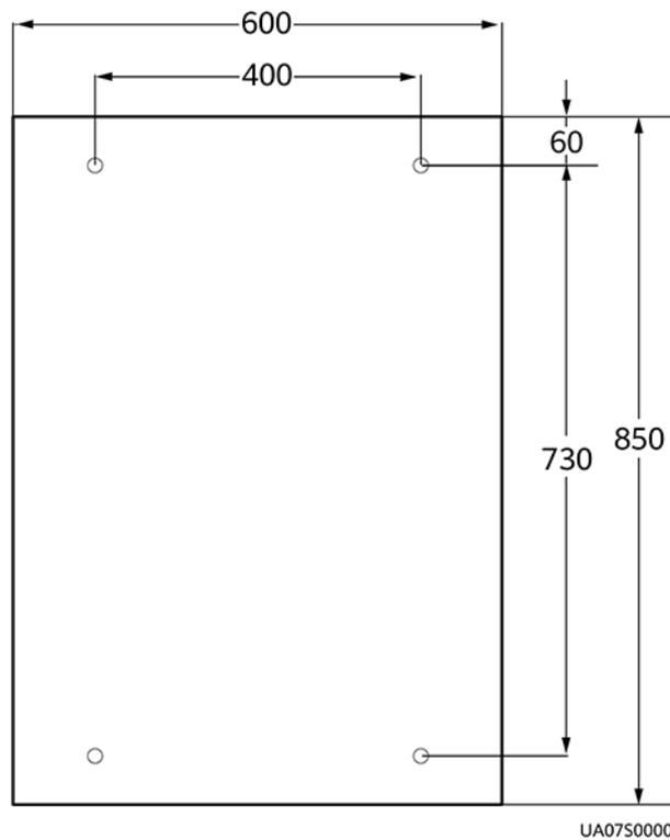
**Step 2** Use a hammer drill to drill four holes for installing expansion bolts and then install four expansion bolts in the holes. **Figure 3-7** shows the composition of an expansion bolt, and **Figure 3-8** shows how to install an expansion bolt.
