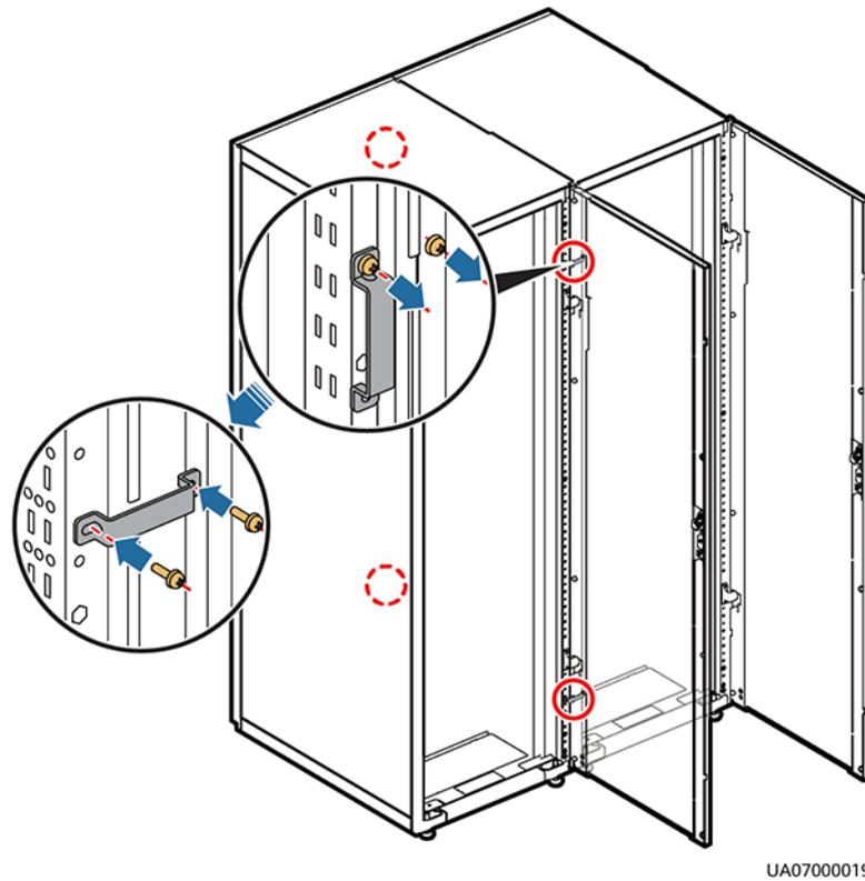
**Figure 3-114** Installing connecting kits (UPS5000-E-200K-FM)
