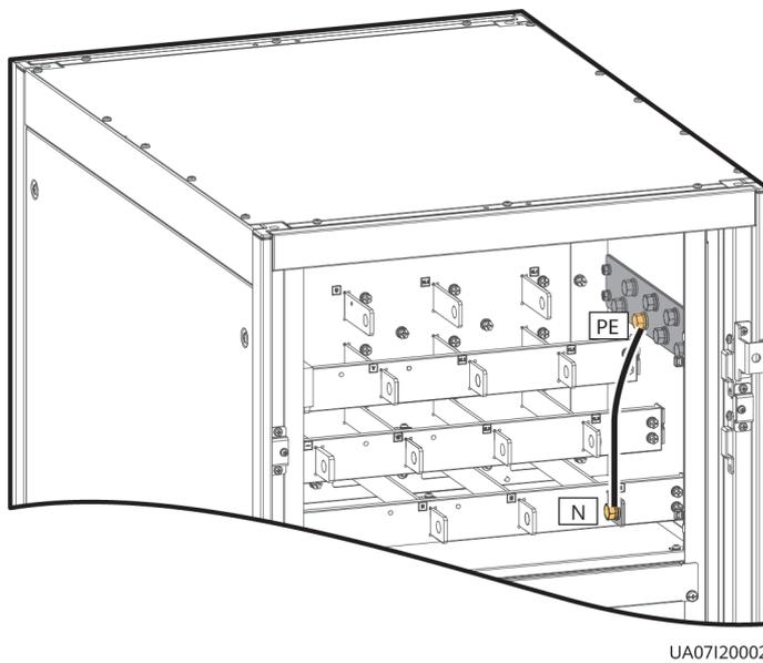
**Figure A-4** Connecting the input N and PE (UPS5000-E-300K-SM)
