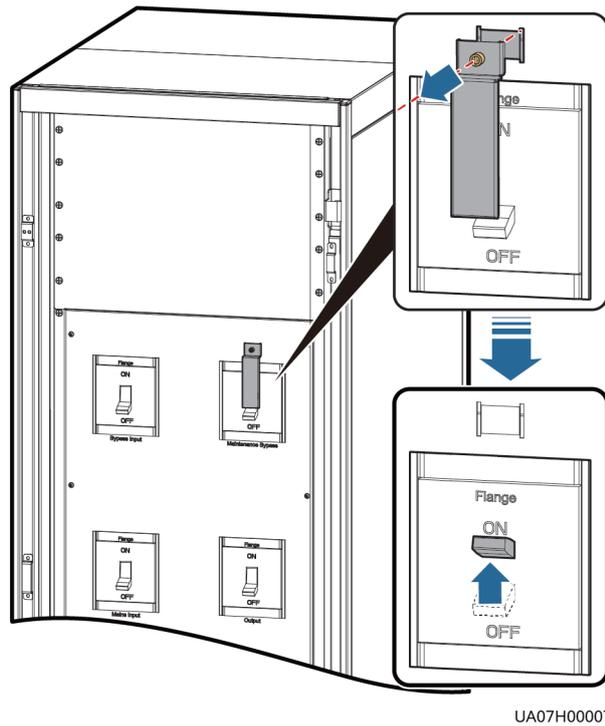
**Figure 8-3** Turning on the maintenance bypass switch (UPS5000-E-200K-FM, isolation protection)
