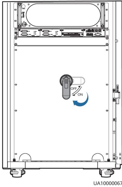
**Figure 8-2** Turning on the maintenance bypass switch (UPS5000-E-200K-FM)
