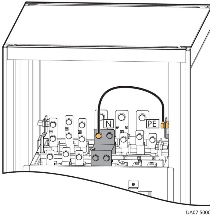
**Figure A-3** Connecting the input N and PE (UPS5000-E-200K-FM, isolation protection)
