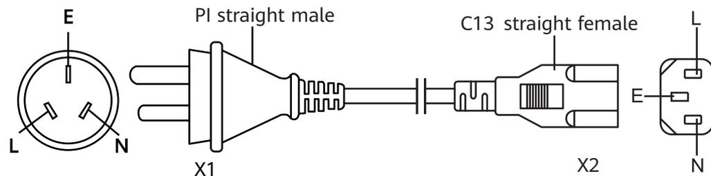
**Figure 5-19** Structure of a Cord end to C13 straight female AC power cable (used in China)
