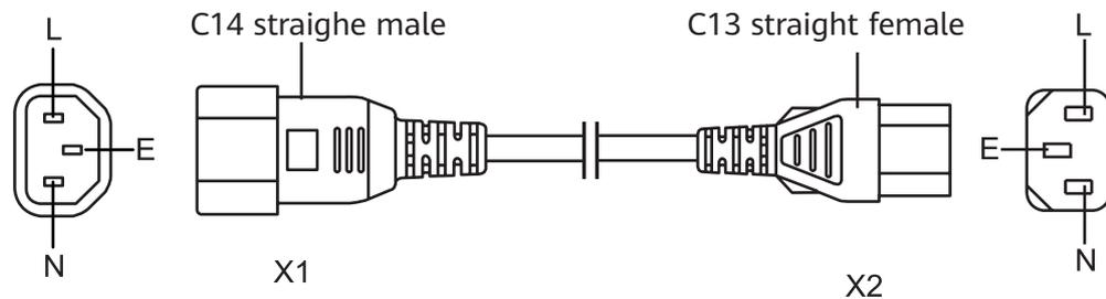
**Figure 5-18** Structure of a PI straight male to C13 straight female AC power cable (used in China)
