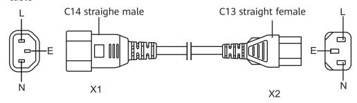
**Figure 5-18** Structure of a PI straight male to C13 straight female AC power cable (used in China)
