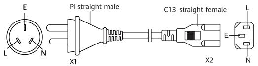
**Figure 5-19** Structure of a Cord end to C13 straight female AC power cable (used in China)
